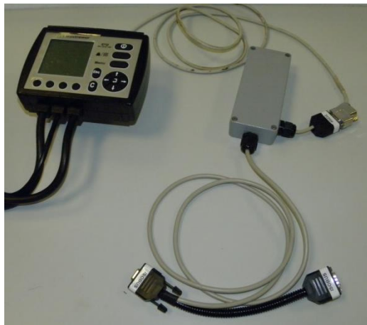
TJ500 with interface device serial / ISOBUS
