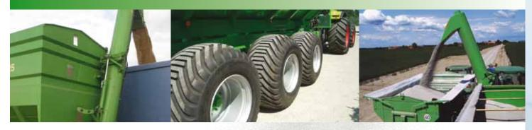
Large windows at the front of the hopper allow the operator full view of the bin loading, optional cameras in the bin and on the unloading auger help with this and the unloading operation. Large diameter wheel equipment ensures minimum ground pressure conditions, a smooth ride and a low rolling resistance resulting in low tractor fuel consumption. The unloading height of up to 4.70m allows a safe transfer loading on slopes or to accommodate differences between field and road height.
